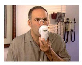
Figure 3. Individual RMR assessment using the MedGem<sup>®</sup> handheld indirect calorimeter.
